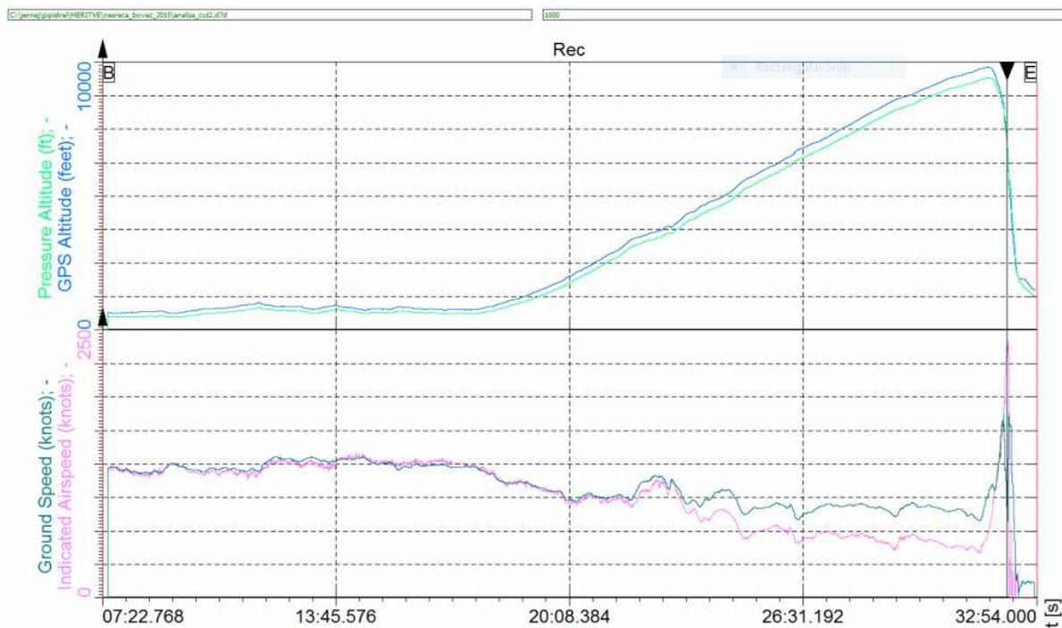
At the time of flight, the cloud base was overcast between (1000-1300 m) 3000-4000 ft. In Instrumental Meteorological Conditions (IMC) and reaching approximately (3000 m) 9800 ft inside clouds where the temperature was 2 degrees Celsius, the aircraft stalled, departed controlled flight and entered a steep dive.
